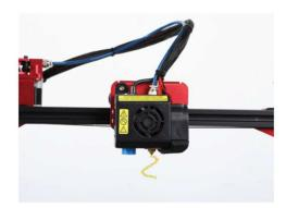
Press and hold the extruder lever and insert the 1.75mm filament through the filament detector and through the extruder motor. Continue feeding until you see filament extrude from the nozzle.
